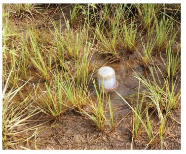
Driver makes Tapered Pilot hole, matching NRU profile. After removal, an NRU is tamped into place
