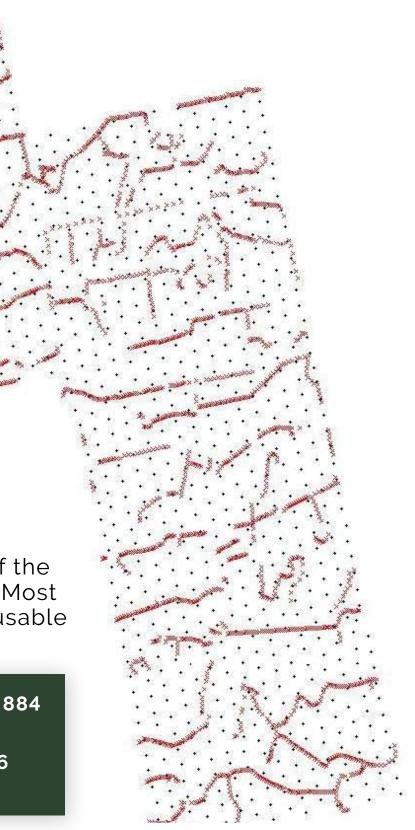
Staggered Receiver spacing, and Near random SPs, eliminate fold patterns induced by standard gridded designs.
